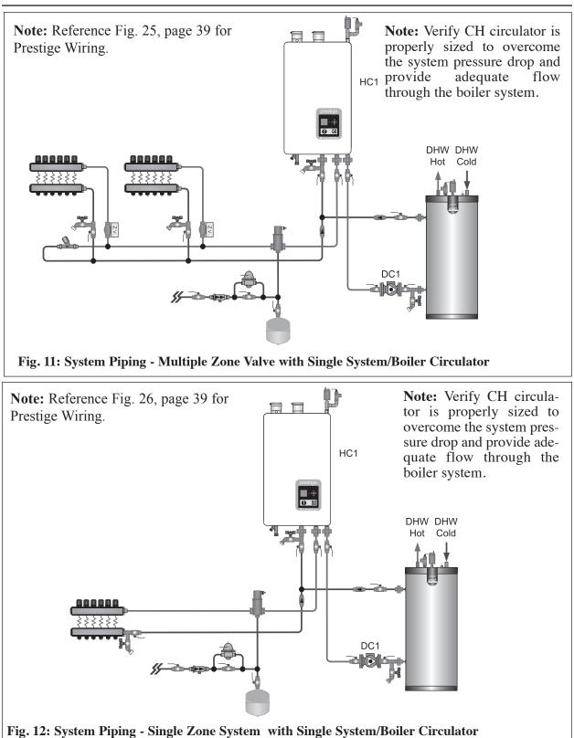
**NOTICE** The boiler system piping shown must be a "closed" system to avoid any oxygen contamination and potential failure of the outer tank of the Smart.
