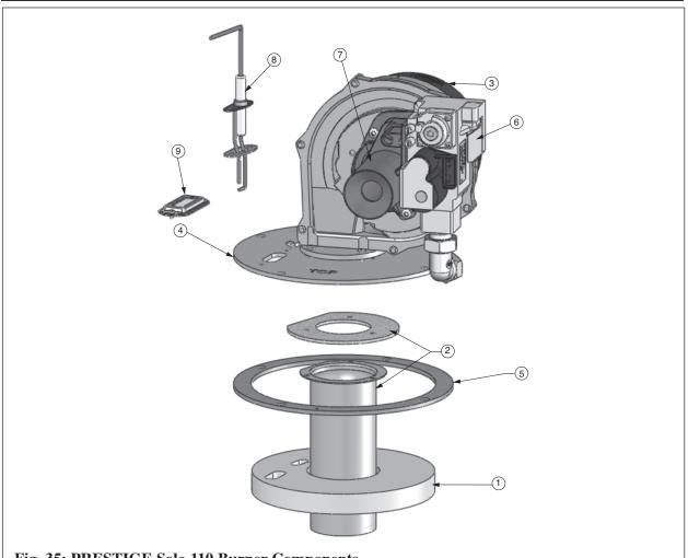
Fig. 35: PRESTIGE Solo 110 Burner Components
